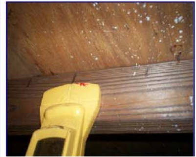
A metal detector is used to determine the nail spacing along the trusses.
