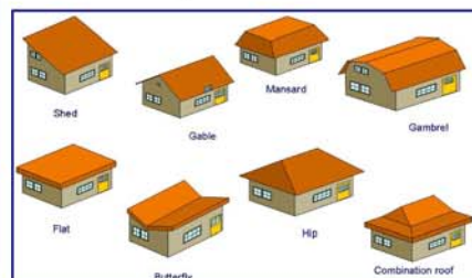
The diagram above shows multiple roof shapes.
