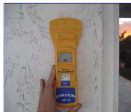
This photo shows the inspector validating the reinforcement in the walls with his metal detector.
